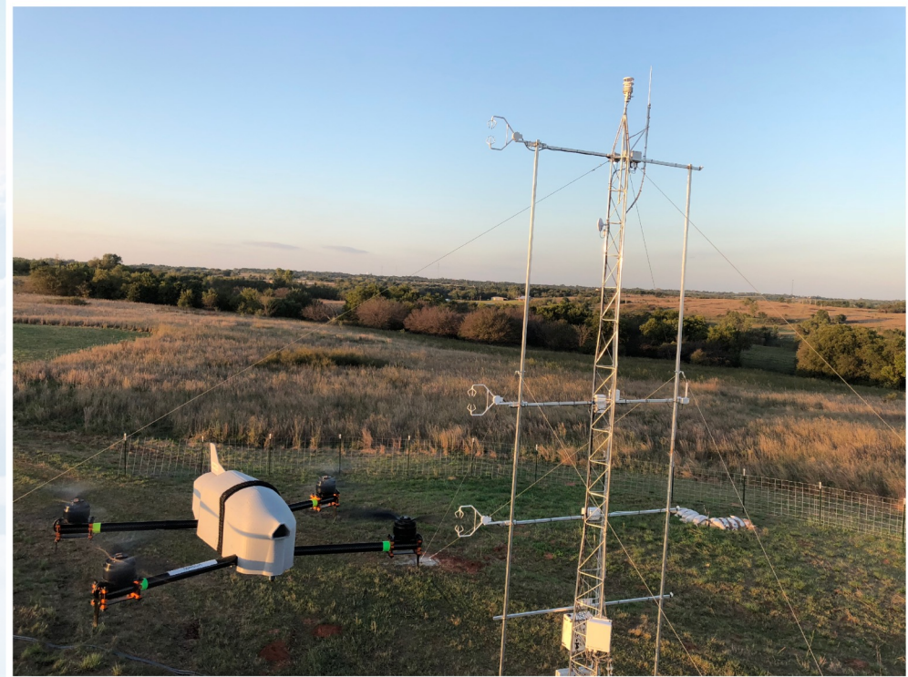
OU CopterSonde (Chilson et al. 2019, Sensors )
