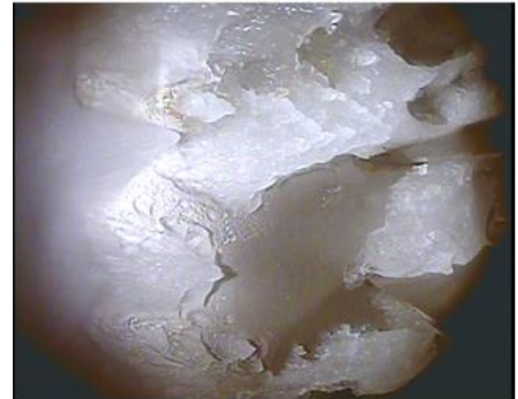
Location of UIAS's and irregular ice accretion seen for full roll back (Escort reading 93)
