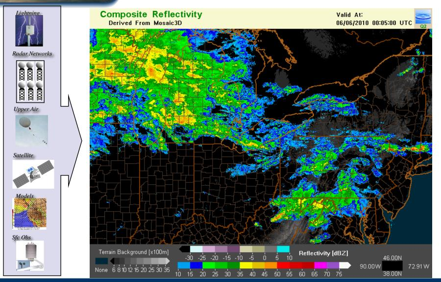
Integrated multiple sensor approach to high resolution rendering of storms and weather
