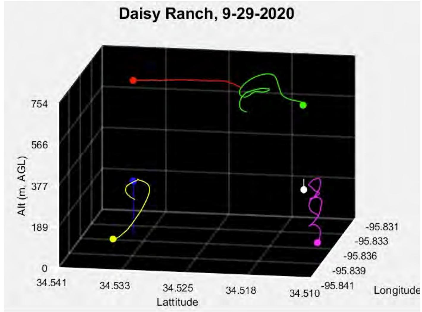
6 Vehicle Autonomous Hybrid One-to-Many to 2,500' Under Part 107
