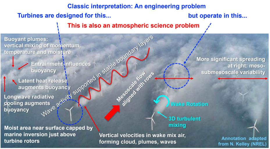
Image from Horns Rev Wind Farm in the North Sea showing turbine wakes. Mesoscale and microscale processes interact. Mesoscale weather and environmental drivers are critical to a full understanding and control of wind plant phenomena.
