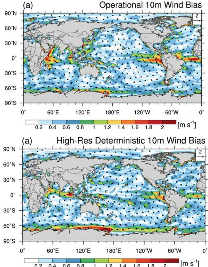
Deterministic 10-m wind speed biases (shading) and wind vector errors (vectors) for operational NAVGEM (top) and Navy ESPC (bottom) averaged for the first 7 days as verified against ECMWF analysis.
