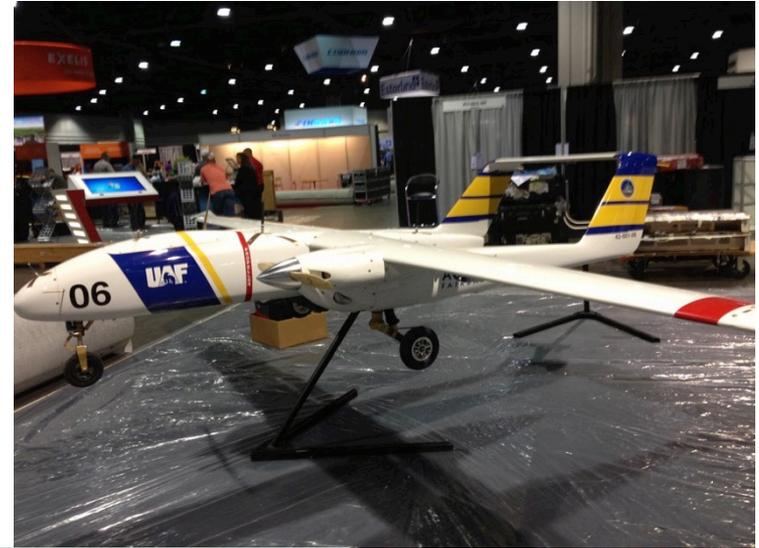
Counter-rotating propellers, heated pitot tubes, fuel injected engines, battery-warmers, and insulation
