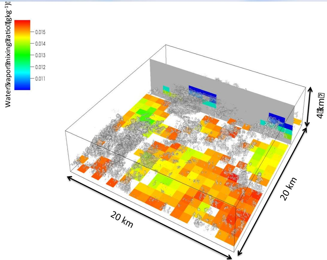
Results from a large-eddy simulation of a cumulus show the key characteristics of the measurements proposed: A differential absorption radar on LEO provides water vapor profiles within cloudy areas along a 'curtain' (grey in figure) with resolution on the order  $1.0 \times 1.0 \times 0.5 \text{ km}^3$ . An IR sounder provides the 3D context of temperature and water vapor structure by sampling the adjacent clear sky regions with resolution of order  $1 \times 1 \text{ km}^2$ .
