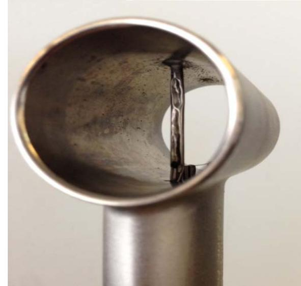
*Lightening strike - in at nose boom, out at trailing edge of IKP*
