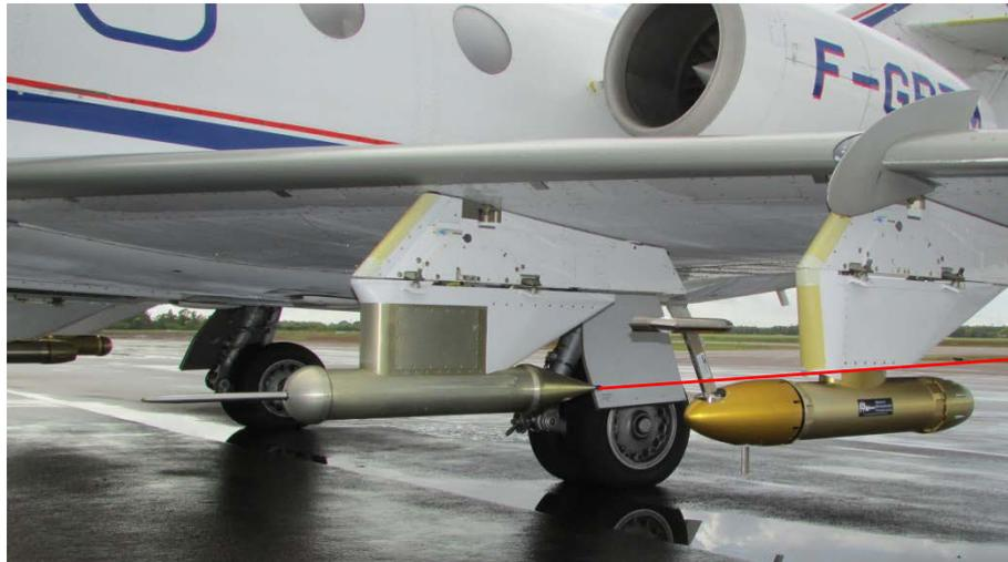
*Erosion damage - radome, wing tip, & LWC sensor*
