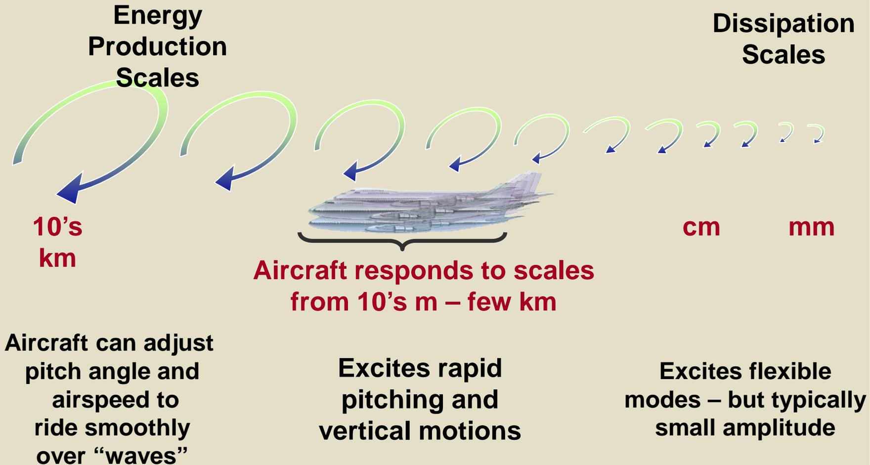
**Aircraft acceleration is a function of the wind spectrum and aircraft response function.**
