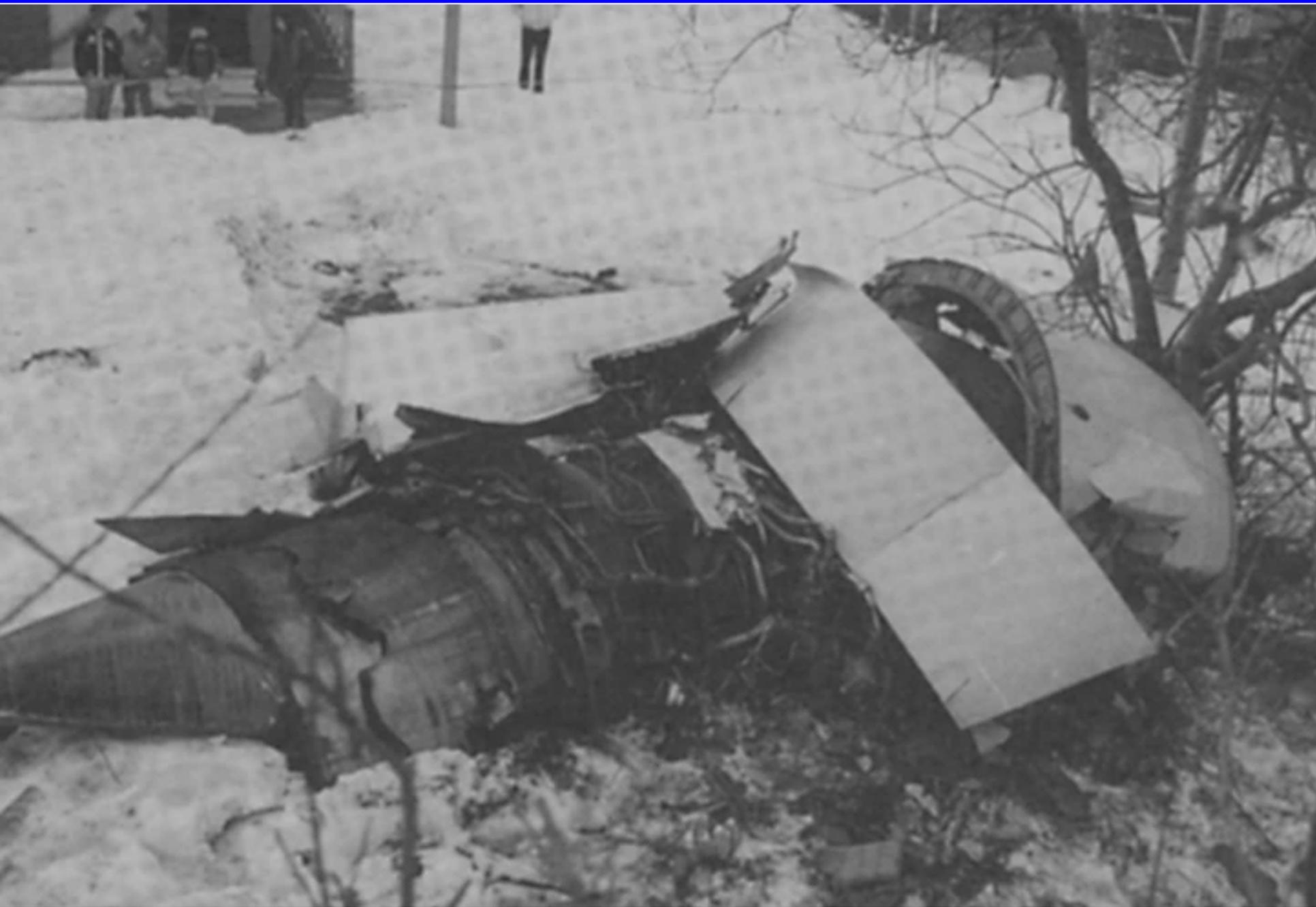
**Evergreen B747 engine after it separated due to turbulence**
