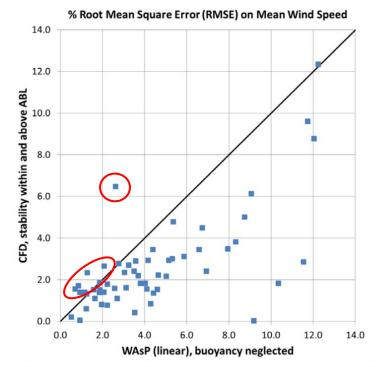
Figure 8 - %RMS error on MWS predictions at each of 57 wind sites, CFD vs. WAsP.
