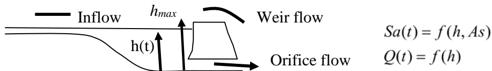
Figure 3.10 Schematic of Level Pool Routing
