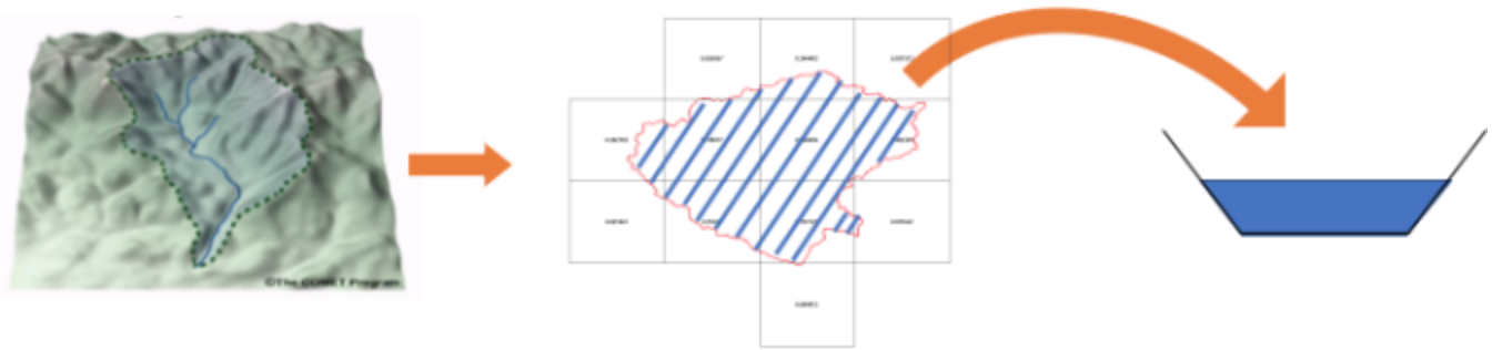
Figure 3.3. An illustration of implementing user-defined mapping to translate from gridded fluxes and states to aggregated catchment fluxes and states, which can be passed into, for example, vector-based channel routing modules.
