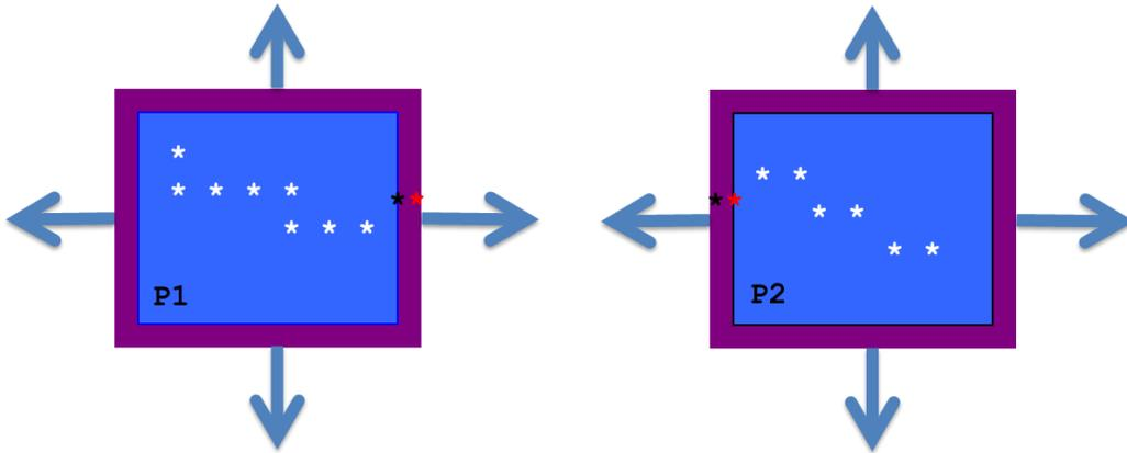
**Figure 2.2** Schematic of parallel domain decomposition scheme in WRF-Hydro as applied to channel routing. Channel elements (stars) are communicated at boundaries via ‘halo’ arrays in which memory is shared between processors (P1 and P2). Black and red stars indicate overlapping channel elements used in the diffusive wave solver.
