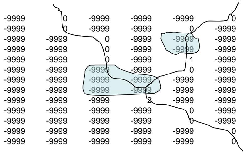
**Figure 4.1** Example of final channel grid format with 2 lake objects present. Note that the main channel identifier index is 0 but that this number changes at lake/reservoir outlet to correspond with the index value of each reservoir shown in Figure 4.2 below. Also, all channel grid cells underneath a lake are assigned as -9999.
