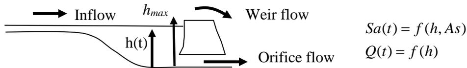
**Figure 3.6** Schematic of Level Pool Routing
