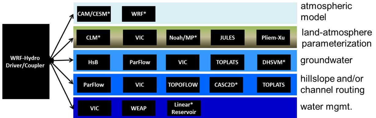
**Figure 1.2.** Model schematic illustrating where many existing atmosphere, land surface and hydrological model components *could* fit into the WRF-Hydro architecture. NOTE: Not all of these models are currently coupled into WRF-Hydro at this time. This schematic is meant to be illustrative. Components which are coupled have an asterisk (\*) by their name.
