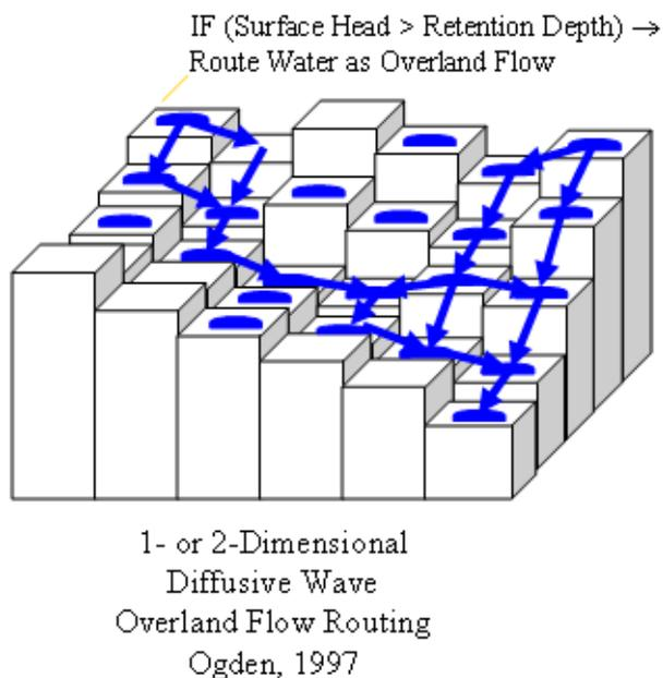
**Figure 3.1: Overland flow outing modules in Noah-d**
