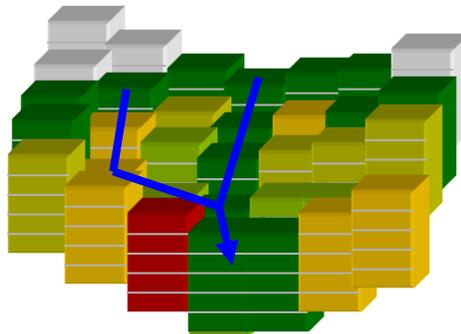
**Figure 3.4:** Conceptual representation of terrain elements. Flow is routed across terrain elements until it intersects a “channel” grid cell indicated by the blue line where it becomes ‘in-flow’ to the stream channel network.
