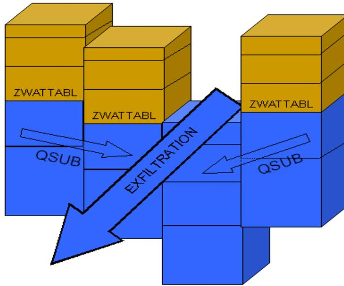
**Figure 3.3 Conceptualization of saturated subsurface flow components.**
