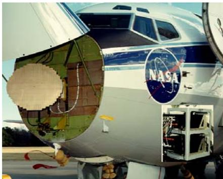
**Forward Looking Turbulence Radar**
