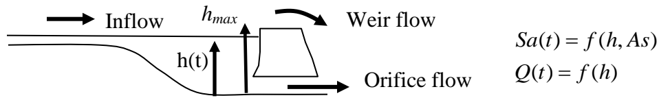
Figure 3.6 Schematic of Level Pool Routing
